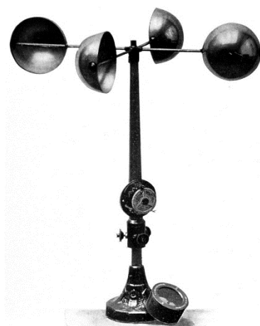
THE ROBINSON ANEMOMETER.
