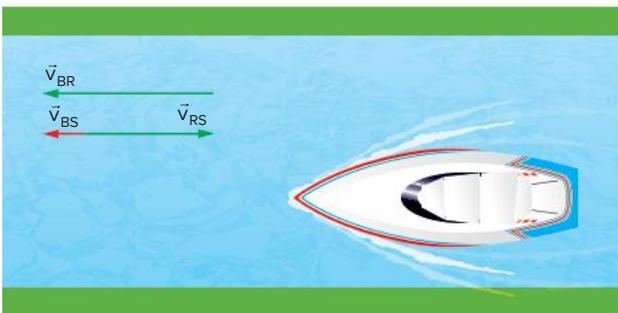
$$|\vec{v}_{BS}| = |\vec{v}_{BR}| - |\vec{v}_{RS}| = 4 \text{ m/s} - 3 \text{ m/s} \Rightarrow |\vec{v}_{BS}| = 1 \text{ m/s}$$
