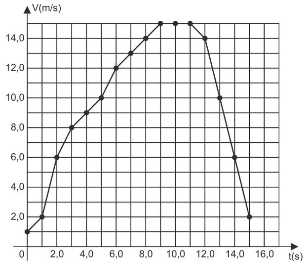
$$(1) \text{ Para } t = 4,0\text{s, temos: } \gamma_1 = \frac{\Delta V_1}{\Delta t_1} = \frac{10,0 - 8,0}{5,0 - 3,0}$$
