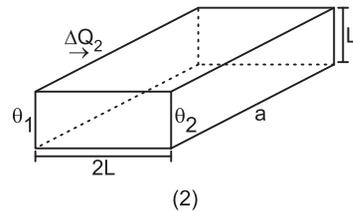
$$\Delta Q_2 = \frac{C S_2 \Delta \theta \Delta t_2}{L_2} \Rightarrow \Delta Q_2 = \frac{C a L \Delta \theta \cdot \Delta t_2}{2L}$$
