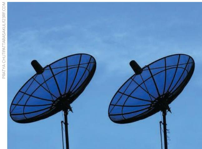
Fig 1 Antena parabólica com receptor no foco principal
