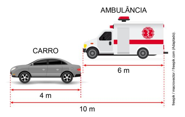
$$\Delta t = \frac{\Delta L}{v_{rel.}} = \frac{10}{10} = 1 \text{ s}$$
