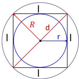
$$\left\{ \begin{array}{l} r = a = \frac{l}{2} \\ d = 2R \\ d = l\sqrt{2} \\ R = \frac{d}{2} = \frac{l\sqrt{2}}{2} \\ A = l^2 \\ 2p = 4l \end{array} \right.$$
