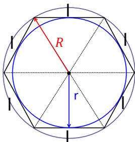
$$\left\{ \begin{array}{l} r = a = \frac{l\sqrt{3}}{2} \\ R = l \\ d = 2r = l\sqrt{3} \\ A = 6 \left( \frac{l^2\sqrt{3}}{4} \right) \\ 2p = 6l \end{array} \right.$$
