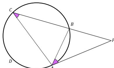
$$(\overline{PA})^2 = \overline{PB} \cdot \overline{PC}$$
