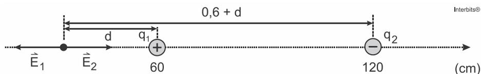
$$E_1 = E_2 = \frac{k|q_1|}{d^2} = \frac{k|q_2|}{(0,6 + d)^2} \Rightarrow \frac{10^{-6}}{d^2} = \frac{4 \times 10^{-6}}{(0,6 + d)^2} \Rightarrow \frac{1}{d^2} = \frac{4}{(0,6 + d)^2} \Rightarrow$$
