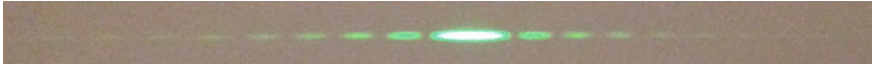
Fig. 5.25 Photo of the diffraction pattern of a slit under Fraunhofer conditions with monochromatic laser light at \lambda = 532 nm. The width of the slit was 50\ \mu\text{m} . No lens was used and the screen was at 2.45 m from the slit. Photo by A. Bettini
