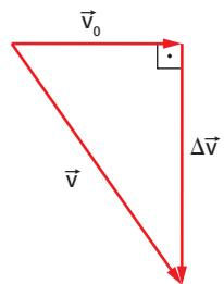
$$\left(\frac{5}{3} |\vec{v}_0|\right)^2 = |\vec{v}_0|^2 + |\Delta \vec{v}|^2 \Rightarrow \frac{25}{9} v_0^2 = v_0^2 + 20^2 \Rightarrow \frac{16}{9} v_0^2 = 20^2 \Rightarrow \frac{4}{3} v_0 = 20 \Rightarrow v_0 = 15 \text{ m/s}$$
