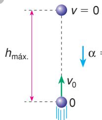
$$h_{\text{máx.}} = \frac{v_0^2}{2g} \Rightarrow \begin{cases} (h_{\text{máx.}})_{\text{Terra}} = \frac{v_0^2}{2g_T} \\ (h_{\text{máx.}})_{\text{Lua}} = \frac{v_0^2}{2g_L} \end{cases}$$
