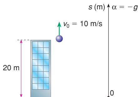
c)  $s = 20 + 10t - 5t^2 \Rightarrow h_{\max.} = 20 + 10 \cdot 1 - 5 \cdot 1^2 \Rightarrow h_{\max.} = 25 \text{ m}$
