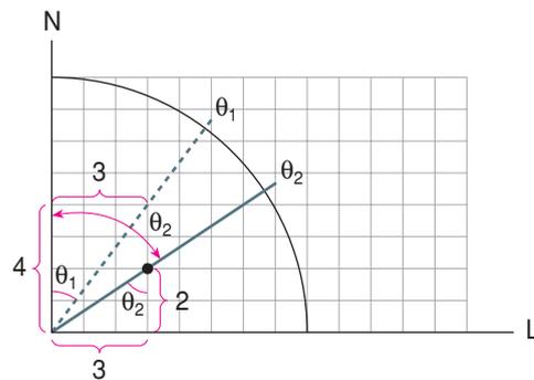
$$\text{tg } \theta_1 = \frac{B_1}{B_T} \Rightarrow \frac{3}{4} = \frac{B_1}{0,2} \Rightarrow B_1 = 0,15 \text{ gauss}$$
