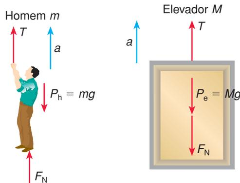
$$\left. \begin{array}{l} \text{Homem:} \\ \text{Elevador:} \end{array} \right\} \begin{array}{l} F_N + T - mg = ma \\ T - F_N - Mg = Ma \end{array} \quad \ominus$$
