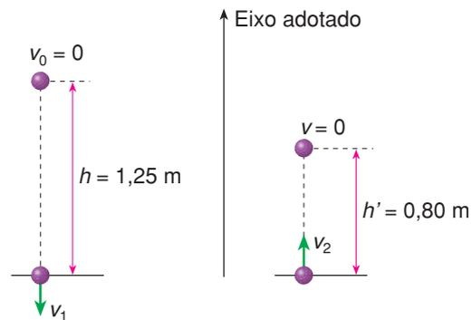
b)  $v_1 = \sqrt{2gh} \Rightarrow v_1 = \sqrt{2 \cdot 10 \cdot 1,25} \Rightarrow v_1 = 5,0 \text{ m/s}$
