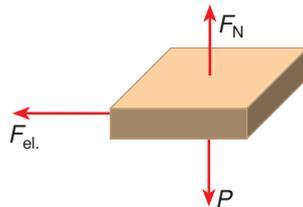
$$b) F_{el.} = m\omega^2 R \Rightarrow kx = m\omega^2 R \Rightarrow k(R - L) = m\omega^2 R \Rightarrow$$
