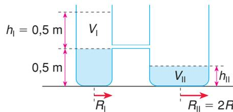
$$V_I = V_{II} \Rightarrow \pi R_I^2 h_1 = \pi R_{II}^2 h_{II} \Rightarrow R_I^2 \cdot 0,5 = (2R_I)^2 \cdot h_{II} \Rightarrow h_{II} = 0,125 \text{ m}$$
