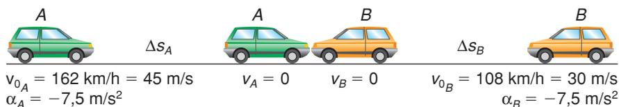
$$v_A^2 = v_{0A}^2 + 2\alpha_A\Delta s_A \Rightarrow 0 = (45)^2 + 2 \cdot (-7,5) \cdot \Delta s_A \Rightarrow \Delta s_A = 135 \text{ m}$$
