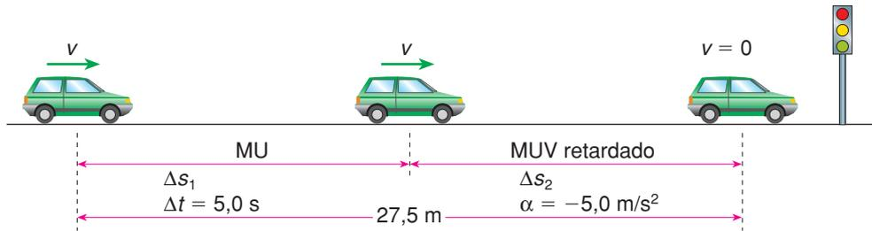
Cálculo de  $\Delta s_1$  (MU):  $v = \frac{\Delta s_1}{\Delta t} \Rightarrow v = \frac{\Delta s_1}{5,0} \Rightarrow \Delta s_1 = 5,0v$
