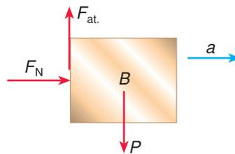
$$F_{at.} = \mu \cdot F_N \Rightarrow P = \mu ma \Rightarrow mg = \mu ma \Rightarrow a = \frac{g}{\mu} \Rightarrow a = \frac{10}{0,9} \text{ m/s}^2 \quad \textcircled{2}$$
