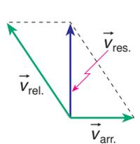
$$\begin{cases} |\vec{v}_{res.}|^2 = |\vec{v}_{rel.}|^2 - |\vec{v}_{arr.}|^2 = 5^2 - 3^2 \\ |\vec{v}_{res.}| = 4 \text{ km/h} \\ \Delta t_{AB} = \frac{AB}{|\vec{v}_{res.}|} \Rightarrow \Delta t_{AB} = \frac{8 \text{ km}}{4 \text{ km/h}} \Rightarrow \Delta t_{AB} = 2 \text{ h} \end{cases}$$
