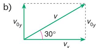
$\text{tg } 30^\circ = \frac{v_{0y}}{v_x} \Rightarrow \frac{\sqrt{3}}{3} = \frac{7,0}{v_x} \Rightarrow v_x = 7,0 \cdot \sqrt{3} \text{ m/s}$
