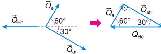
$$\text{sen } 60^\circ = \frac{Q_{an.}}{Q_{He}} \Rightarrow \frac{\sqrt{3}}{2} = \frac{Q_{an.}}{12 \cdot 10^{-24}} \Rightarrow Q_{an.} = 6,0\sqrt{3} \cdot 10^{-24} \text{ kg} \cdot \text{m/s}$$
