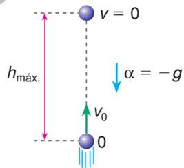
$$h_{\text{máx.}} = \frac{v_0^2}{2g} \Rightarrow \begin{cases} (h_{\text{máx.}})_{\text{Terra}} = \frac{v_0^2}{2g_{\text{T}}} \\ (h_{\text{máx.}})_{\text{Lua}} = \frac{v_0^2}{2g_{\text{L}}} \end{cases}$$
