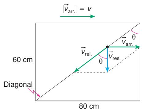
$$\begin{aligned} \text{tg } \theta &= \frac{|\vec{v}_{arr.}|}{|\vec{v}_{res.}|} \\ \frac{80}{60} &= \frac{v}{v_g} \\ v_g &= \frac{3}{4}v \end{aligned}$$
