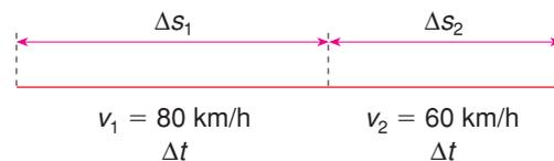
$$v_m = \frac{\Delta s_{\text{total}}}{\Delta t_{\text{total}}} \Rightarrow v_m = \frac{v_1 + v_2}{2} \Rightarrow v_m = \frac{80 + 60}{2} \Rightarrow v_m = 70 \text{ km/h}$$
