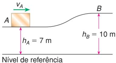
$$E_{\text{mec.}(A)} = E_{c(A)} + E_{p(A)} = \frac{mv_A^2}{2} + mgh_A$$
