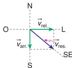
$$v_{res.}^2 = v_{rel.}^2 + v_{arr.}^2$$
