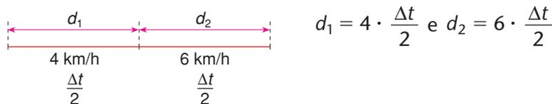
$$v_m = \frac{\Delta s}{\Delta t} \Rightarrow v_m = \frac{d_1 + d_2}{\Delta t} \Rightarrow v_m = \frac{4 \cdot \frac{\Delta t}{2} + 6 \cdot \frac{\Delta t}{2}}{\Delta t} \Rightarrow$$
