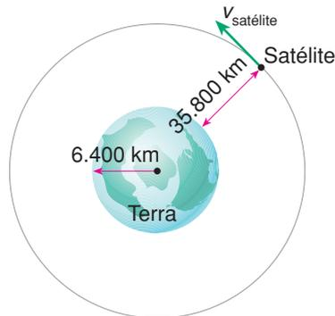
$$\omega_s = \omega_T = \frac{2\pi}{24} \Rightarrow \omega_s = \omega_T = \frac{\pi}{12} \text{ rad/h}$$
