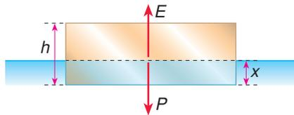
$$P = E \Rightarrow d_p V_p g = d_a V_a g \Rightarrow \frac{d_p}{d_a} = \frac{V_a}{V_p} = \frac{x A}{h A} \Rightarrow \frac{d_p}{d_a} = \frac{0,4}{1,2} = \frac{1}{3} \Rightarrow d_{p,a} = \frac{1}{3}$$
