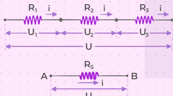
$$R_s = R_1 + R_2 + R_3$$
