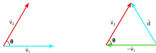
$$d^2 = v_1^2 + v_2^2 - 2v_1 \cdot v_2 \cos \theta \text{ (módulo)}$$
