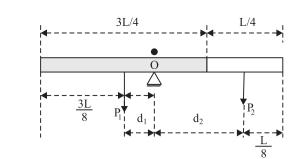
$$\begin{array}{c} L_1 + L_2 = L \\ L_1 = 3L_2 \end{array} \bigg\} \ L_2 = \frac{L}{4} \ e \ L_1 = \frac{3L}{4} \\ \end{array}$$
