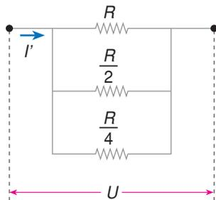
$$\frac{1}{R_{\text{eq.}}} = \frac{1}{R} + \frac{2}{R} + \frac{4}{R} \Rightarrow \frac{1}{R_{\text{eq.}}} = \frac{7}{R} \Rightarrow R_{\text{eq.}} = \frac{R}{7}$$
