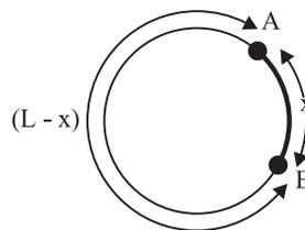
$$r_{AB} = \rho \frac{x}{A} \quad \text{e} \quad R_{AB} = \rho \frac{(L-x)}{A}$$
