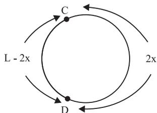
$$r_{CD} = \rho \frac{2x}{A} \quad \text{e} \quad R_{CD} = \rho \frac{(L-2x)}{A}$$
